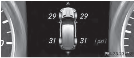
Example: current tire pressure display
