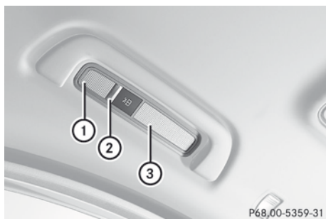
Rear-compartment overhead control panel
